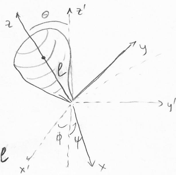
$\theta$  - inclination of the  $z$  axis from the vertical
